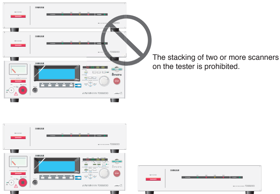
Fig.1-3 Installation of Two Scanners
