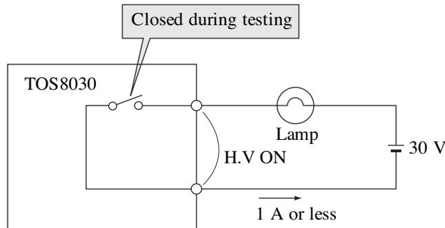
Fig. 7-3 Example: Use of an H.V ON Signal
