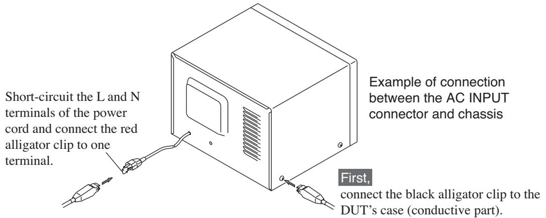
Fig. 3-3 Example of Connection to the DUT
