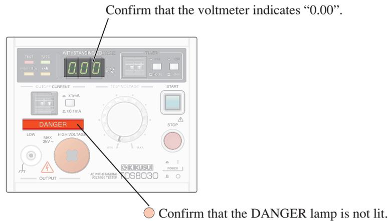
Fig. 3-7 Checking for the Absence of High Voltage
