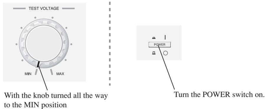
Fig.5-1 Check when Turning the POWER Switch On
