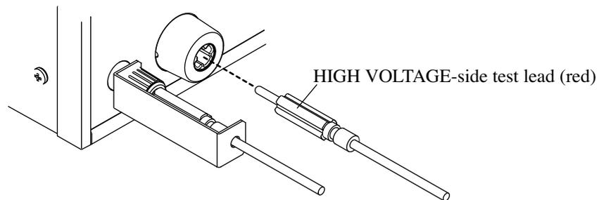
Fig. 3-4 Connecting the HIGH VOLTAGE-side test lead
