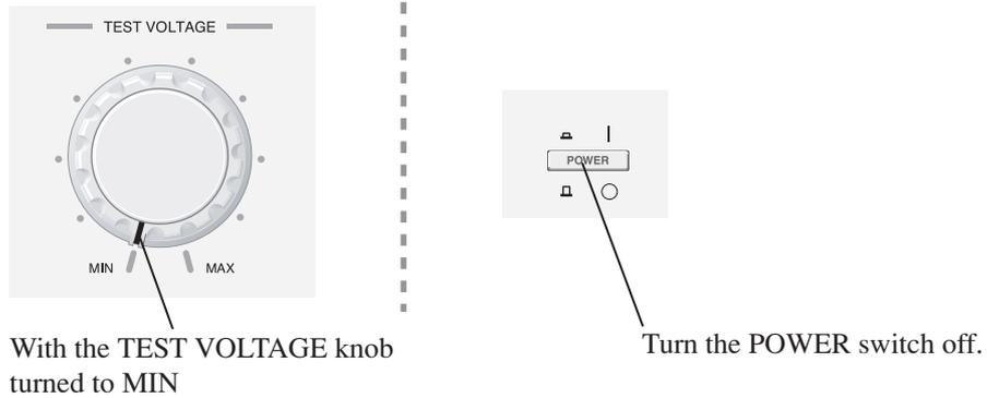
Fig. 3-9 When Interrupting Operations
