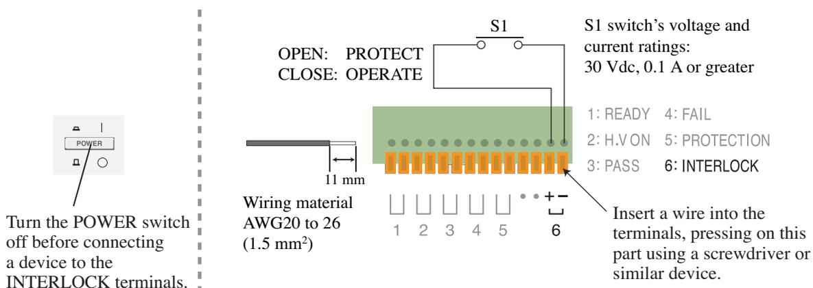
Fig. 6-6 Connecting a Device to the INTERLOCK Terminals
