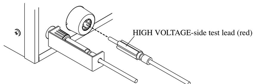
Fig. 3-8 Disconnecting the HIGH VOLTAGE-side Test Lead
