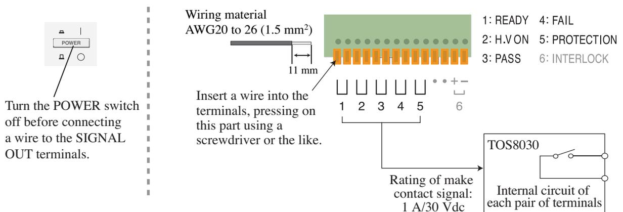
Fig. 7-1 Connecting a Wire to the SIGNAL OUT Terminals
