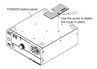
When you want to use the TOS5200 without the protection cover attached, such as when you will repeatedly perform tests with frequently changed test conditions, you can store the protection cover on the product's bottom panel. This is useful in preventing the cover from being lost.
