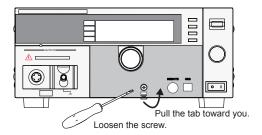
Loosen the screw, and then pull the tab at the bottom center of the cover towards you to remove the protection cover from the panel.
