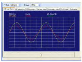
When you have set the standard to IEC Ed4.0/Ed2.1 or IEC Ed4.0/Ed1.0, the class to class C, and the limit values to 3rd/5th/Current Wave, the current waveform analysis diagram that is prescribed from IEC 61000-3-2: Ed3.0 (2005)/A2 (2009) is displayed in place of the V/I waveform in the test results file.
