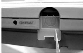
Fig.2-5 Connector Cover Removal
