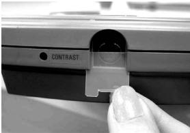
Fig.2-4 Connector Cover Installation
