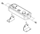
To fix the remote control box, install provided brackets as shown in Figure left.
