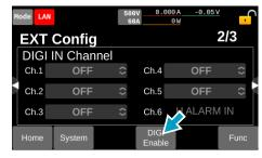
Enable the digital input/output.
