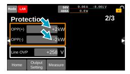
Use the display or the rotary knob to enter the power value.
