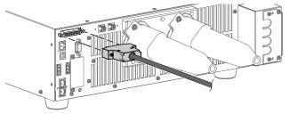
Connect the signal cable to the external controller.
