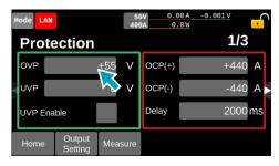
3 Use the display or the rotary knob to enter the voltage value.
