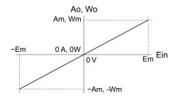
Ao: Output current Wo: Output power Am: Rated current  $-Am \le Ao \le Am$   $-Wm \le Wo \le Wm$ Wm: Rated power Ein: External voltage Em: 5 V or 10 V
