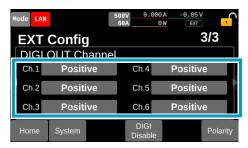
If the input field is grayed out, press DIGI Enable to enable the digital input/output. This completes the setting.
