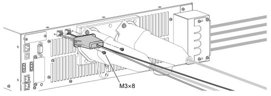
6 Connect the sensing cables to the DUT.
