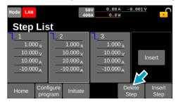
• Press Delete in the state where the multiple steps are pressed and selected by holding down the steps on the step list screen.
