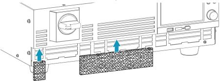
Attach the dust filters to the inside of the louver.
