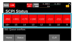
The details of the error will be displayed under the error number. The details of the error will be displayed. For details on errors, see the Communication Interface Manual on the included CD-ROM.
