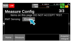
When remote sensing is enabled, the sensing icon ( $\frac{4}{2}$ ) appears on the upper right part of the display.
