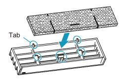
Attach the louver to the front panel.
