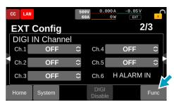
It switches in the order of "Func"  $\rightarrow$  "Filter"  $\rightarrow$  "Polarity" to display the polarity setup screen for each channel.
