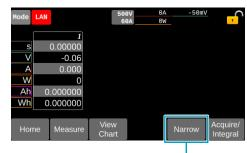
Switching between detailed and simplified displays
