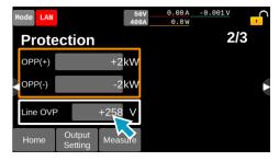
Use the display or the rotary knob to enter the voltage value.
