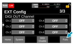
"Func" switches to "Polarity" to display the polarity setup screen for each channel.
