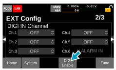
Enable the digital input/output.
