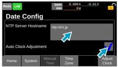
Press the input field for Auto Clock Adjustment and check the box.
