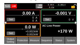
By factory default, the panel settings immediately before the POWER switch is turned off are saved. When you turn the power on, the product starts in the same state as it was in the last time it was turned off.s
