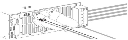
Attach the sensing terminal cover.
