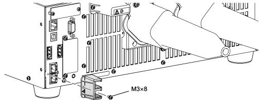
Connect all PXB series with the included synchronized operation signal cables.
