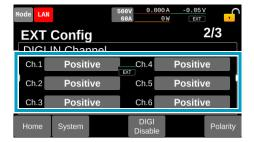
If the input field is grayed out, press DIGI Enable to enable the digital input/output.
