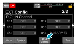
Enable the digital input/output.
