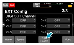
Enable the digital input/output.
