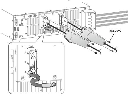
After installing of the OUTPUT terminal cover (Bottom view of the OUTPUT terminal cover)
