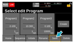
Input the program name with the display or rotary knob and press OK.
