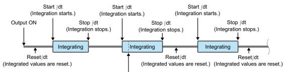
The system records the integrated values at a point in time when the period set in Average of Acquire Trigger has elapsed since the measured value recording is started.
