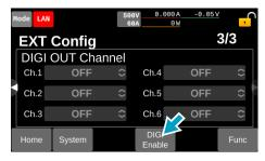
Enable the digital input/output.
