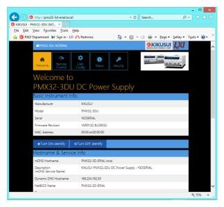
Turn ON Identify: The LAN LED on the front panel of the connected PMX blinks so that you can identify it.
