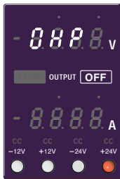
Fig. 2-7 OHP alarm indicator
