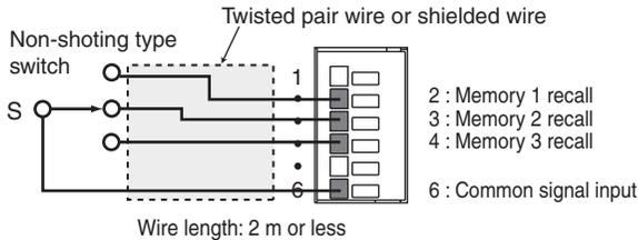
Fig. 5-4 Connecting a contact switches for memory recall 1 (When using a non-shorting type switch)
