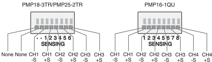
Fig. 4-19 Corresponding remote sensing terminals
