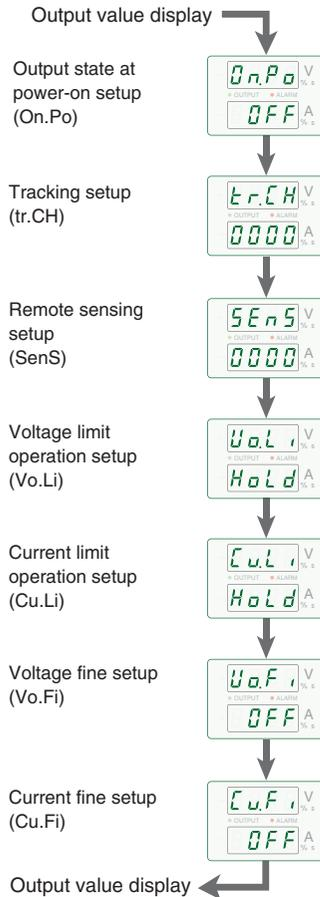
Fig. 4-18 CONFIG settings (Factory-shipped settings)
