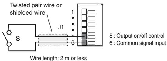
Fig. 5-3 Connecting a contact switches for output on/off
