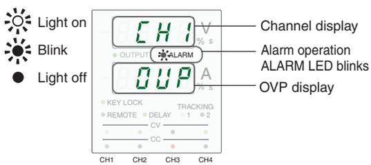
Fig. 4-5 OVP alarm display (example of activation of over-voltage protection in CH1)
