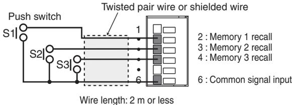
Fig. 5-5 Connecting a contact switches for memory recall 2 (When using push switches)
