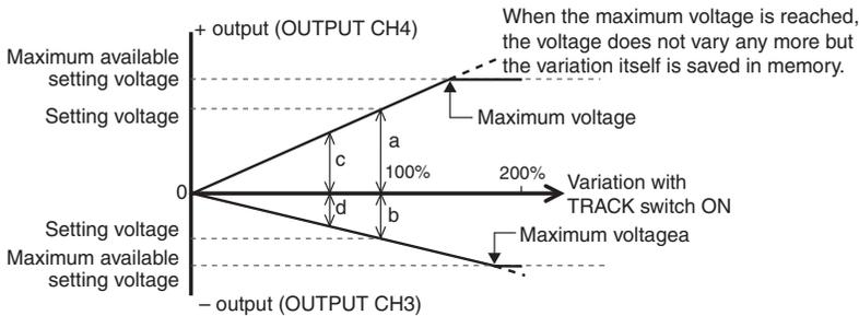
Fig. 4-8 Voltage setting and tracking output
