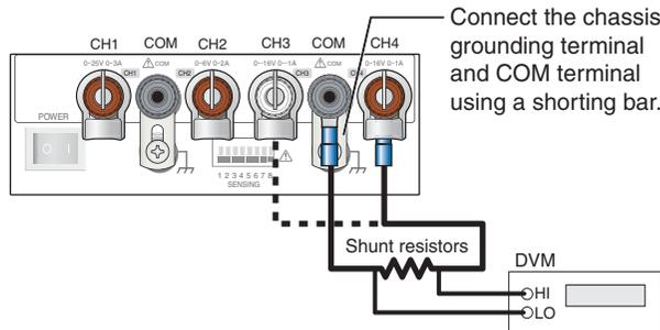
Fig. 6-6 PMP16-1QU current adjustment connection example 2
