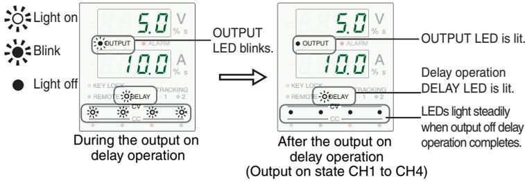
Fig. 4-15 Example of display during output off delay operation
