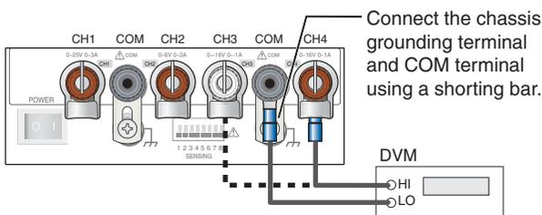
Fig. 6-3 PMP16-1QU voltage adjustment connection example 2
