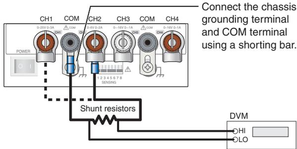
Fig. 6-5 PMP16-1QU current adjustment connection example 1
