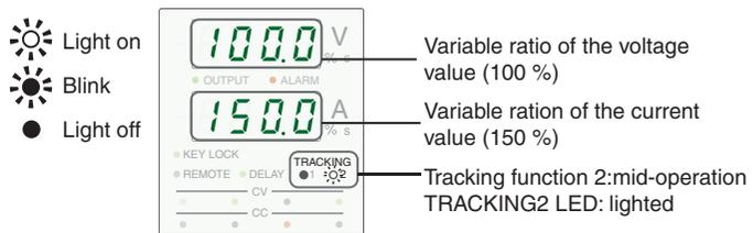
Fig. 4-11 Tracking function 2: Example of display during operation
