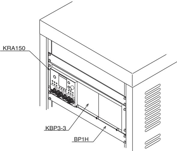
Fig. 1-1 Rack-mounting example
