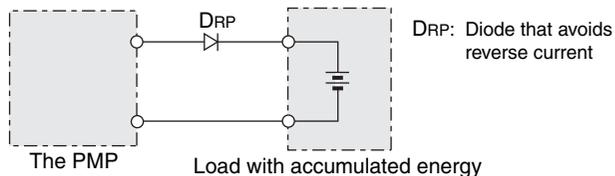
Fig. 3-4 Remedy against load with accumulated energy
