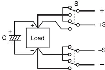
Fig. 4-22 On/off using the mechanical switch
