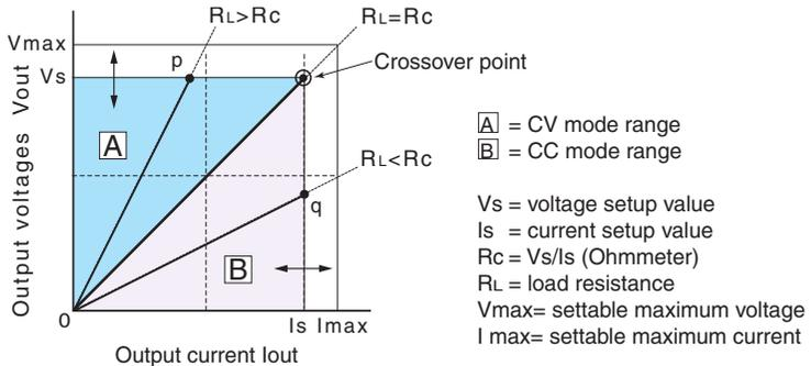
Fig. 4-3 Constant voltage operation and constant current operation
