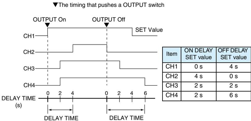
Fig. 4-12 Timing chart of delay function
