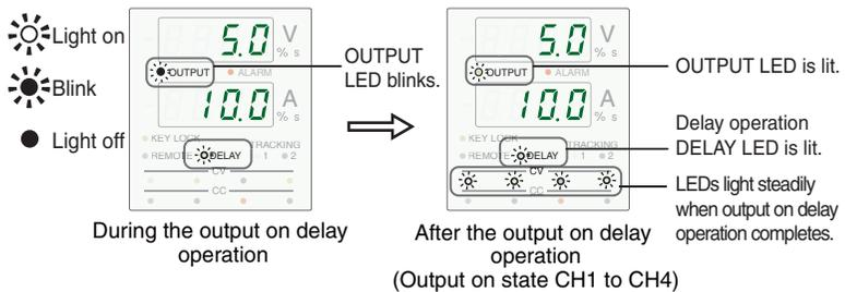
Fig. 4-14 Example of display during output on delay operation
