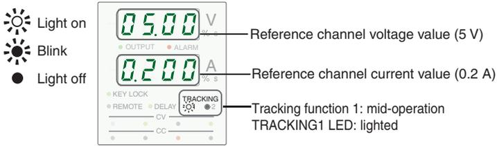
Fig. 4-10 Tracking function 1: Example of display during operation
