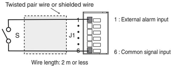
Fig. 5-8 Connecting a contact switch to alarm input
