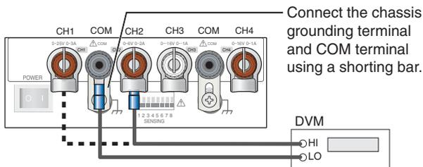
Fig. 6-2 PMP16-1QU voltage adjustment connection example 1
