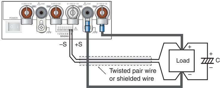
Fig. 4-20 Remote sensing connection example
