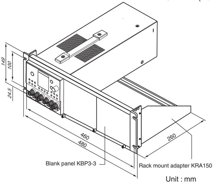
Fig. 1-2 Example of installation options for rack mounting
