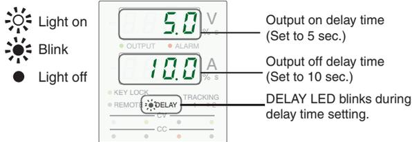
Fig. 4-13 Example of delay time setting display
