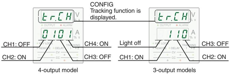
Fig. 4-9 Display example of setting a tracking function
