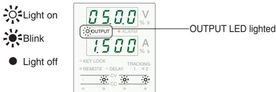
Fig. 4-2 Examples of output on display
