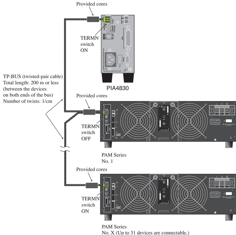
The TP-BUS is connected in a chain by connecting twisted-pair cables to the TP-BUS connectors (plug.) The total length of a twisted-pair cable, when connected to the series, is 200 m or less.
