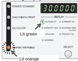
Example of warning indication, 30 V voltage display
