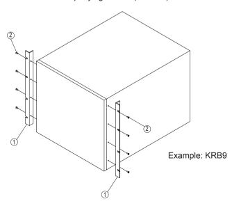
3. Using the accompanying screws and washers, mount the instrument in the rack. Be sure to use the accompanying screws (M5 x 14) and washers.
