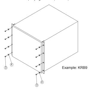
**CAUTION** The instrument may fall. Install the suitable support angles applying to the used rack system to support the instrument.
