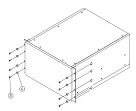
**CAUTION** The instrument may fall. Install the suitable support angles applying to the used rack system to support the instrument.
