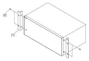
Install the rack mounting unit to the EIA standard rack using the provided screws and washers.
