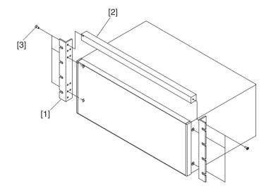
2. Install the rack mounting instrument to the JIS standard rack using the provided screws and washers.
