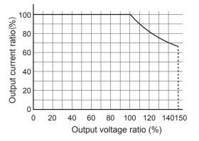
Fig.2 Output voltage ratio versus rated output current ratio (DC mode)
