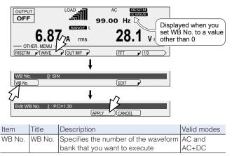
If the output is on, the selected waveform will be generated. If the output is off, press OUTPUT to turn the output on and generate the selected waveform.
