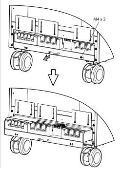
Pull out the stopper to lock the terminal block tray in place.
