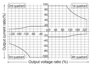
If you use the PCR-LE2 Series with a current that exceeds the rated DC output current, the protection functions will be activated, which may cause the output voltage to drop or turn off the output.
