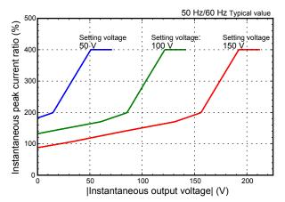
Fig.11 Instantaneous output voltage ratio versus instantaneous peak current ratio (AC mode H range, excluding threephase three-wire output)
