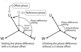
To avoid confusion, we recommend that you turn off the U phase offset when you use the phase sweep feature. For details, see "Phase setting for multi-phase output" in the sequence tutorial of the appendix.
