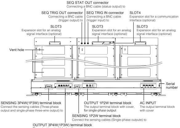
The output terminal block with cover
