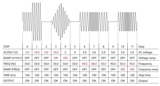
This page explains how to use a sequence to output the following waveform.
