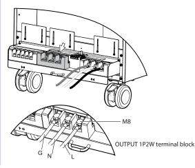
5 Return the terminal block tray to its previous position. If you do not insert the terminal block tray all the way into its storage compartment, an electric current will not flow through the PCR-LE2 Series even if the POWER switch is turned on.
