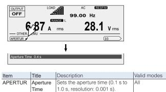
The aperture time setting was added in firmware version 5.00. As a result, the function for averaging measured values that was available in firmware version 4.99 and earlier is no longer available.
