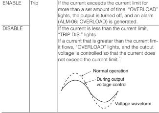
\*1. This is calculated as an rms value. The current limit may be exceeded for a few seconds because of the relationship between the measurement processing time and the voltage resolution. The current may oscillate (increase and decrease) while it is being controlled.
