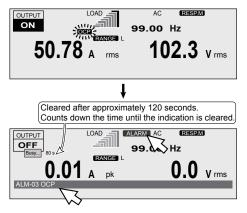
If the internal semiconductor protection is activated repeatedly, the PCR-LE2 Series may malfunction.
