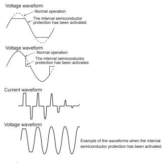
In AC mode, you can set the time that elapses after the internal semiconductor protection function is activated before an alarm is generated. An alarm will only be generated if the internal semiconductor protection function circuit remains activated continually for the specified length of time. This is useful when you don't want alarms to be generated due to short-term overloads such as those caused by inrush current.
