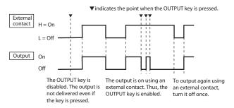
When a sequence is running, the output on/off control through external contacts is invalid.
