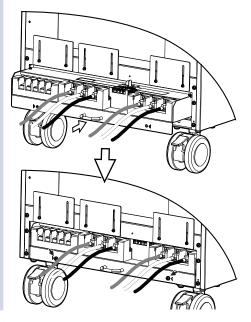
Slide the two terminal box covers down until they are touching the wires, and then use the four screws to fix the terminal box covers in place. Slide the terminal box cover all the way down if none of their terminals have wires connected to them, and use the two screws to fix the covers in place.
