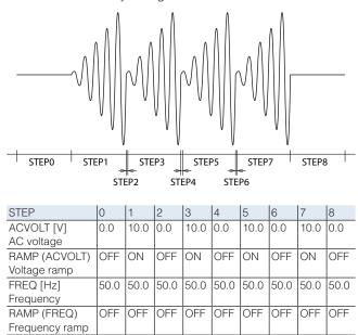
In a step whose ramp is set to on, the voltage changes linearly from the voltage setting of the previous step to the specified voltage.
