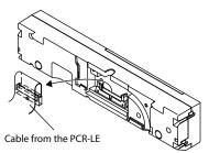
4 Connect the cable from the PCR-LE2 Series to the control panel extension cable. Use the band and the bracket to fix the control panel extension cable to the PCR-LE2 Series.
