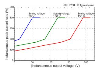
Fig.6 Instantaneous output voltage versus instantenous peak current ratio (AC mode H range, excluding three-phase three-wire output)
