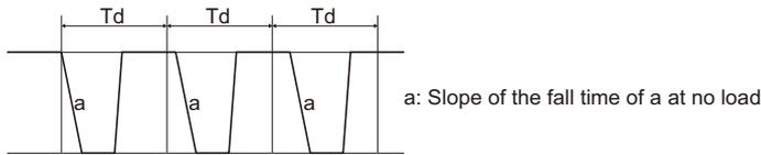
9. Duration for the voltage to change from 90 % to 10 % of the rated output voltage when the output voltage is repeatedly decreased and the duration from a given voltage drop to the next voltage drop is shorter than Td.
