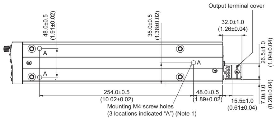
(Note 1) Keep screw insertion depth to 6 mm or less.
