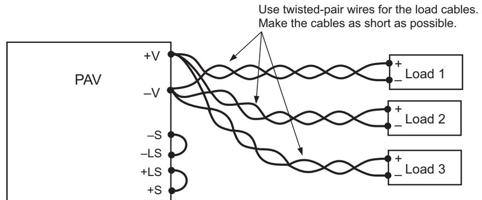
When using sensing cables, connect them to the output terminals of the PAV series or to a single load that you want to reduce the load variation the most.
