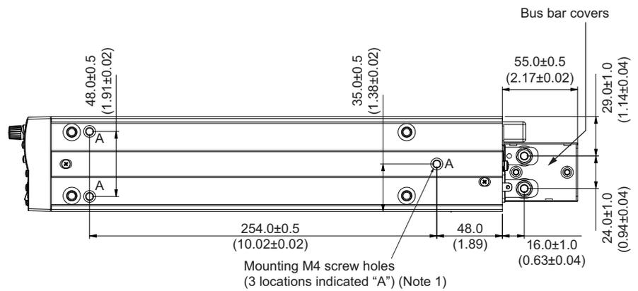
(Note 1) Keep screw insertion depth to 6 mm or less.
