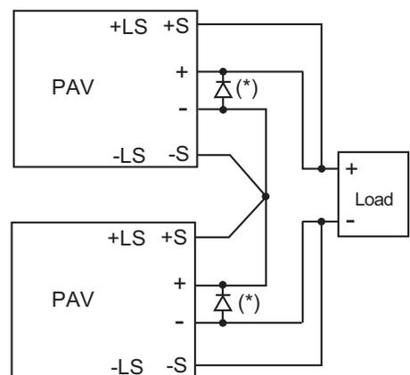
(\*) Connect the diode externally.
