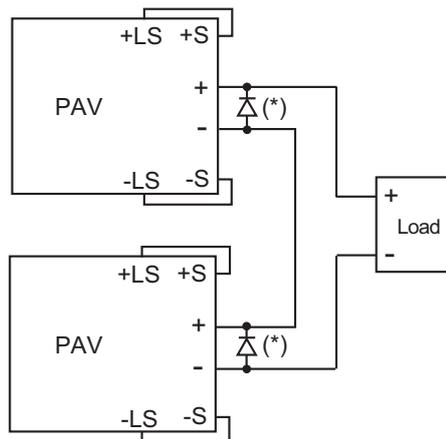
Series connection using remote sensing
