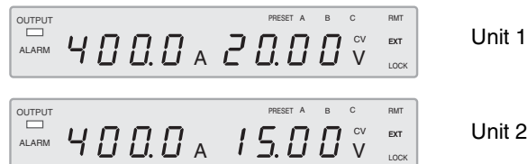
Fig.4-7 Panel display example during series operation
