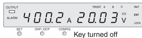
Fig.2-1 Measured value display example
