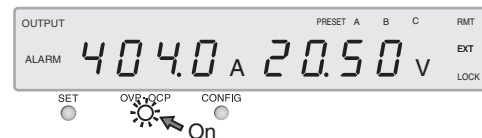
Fig.2-3 Setting display example of the overvoltage and overcurrent protection
