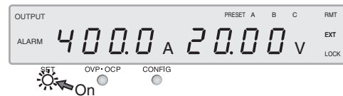
Fig.2-2 Setting display example of the output voltage and output current
