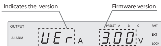
Firmware version display at power-on (example for Ver.3.00)
