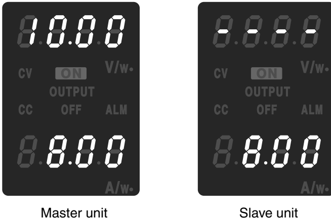
Fig.5-5 Panel display during parallel operation
