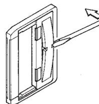
To remove the cover of the handle, put the screw driver in the gap, and twist it.
