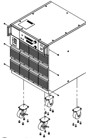
2. As shown in figure, using ④ and ⑤ screws, install ①, ② and ③ brackets.
