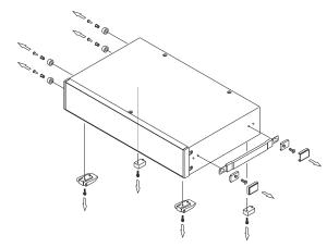
2. As shown in figure, using the accompanying screws, install the brackets. Do not use except the accompanying screws (M3 or M4 x 10 flat screws).
