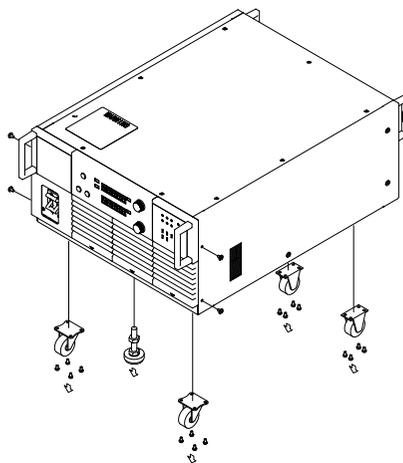
2. As shown in figure, using the accompanying screws, install the brackets. For No.4 screws, do not use except the accompanying screws (M4 x 14 flat head screws).
