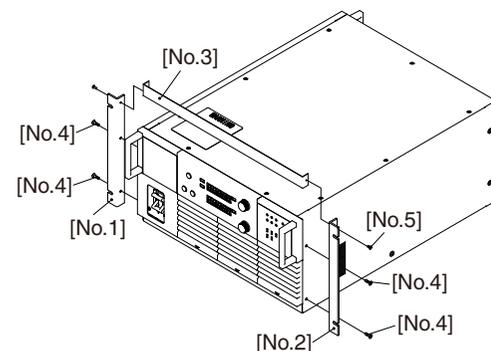
3. Using the accompanying screws and washers, mount the instrument in the rack.
