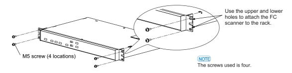
**CAUTION** The instrument may fall. Install the suitable support angles applying to the used rack system to support the instrument.
