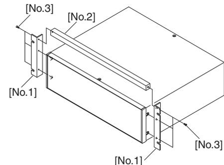
3. Using the accompanying screws and washers, mount the instrument in the rack.
