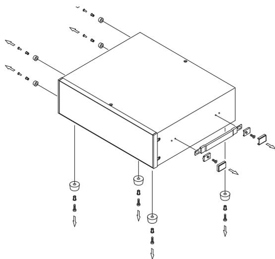
2. As shown in figure, using the accompanying screws, install the brackets. Do not use except the accompanying screws (M4 x 10 flat head screws).
