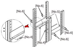
4. Using No.8 screws and No.7 washers, mount the instrument in the rack.
