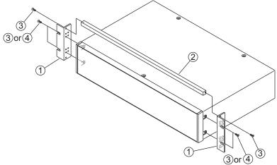
3. Using the accompanying screws and washers, mount the instrument in the rack.
