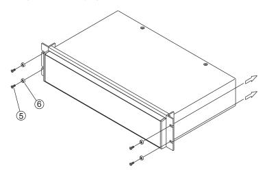
!\CAUTION The instrument may fall. Install the suitable support angles applying to the used rack system to support the instrument.
