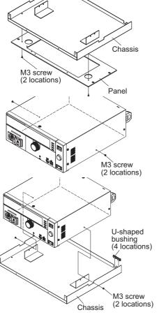
1 Unscrew the M3 screws (M3x8) that are holding the panel and chassis together.
