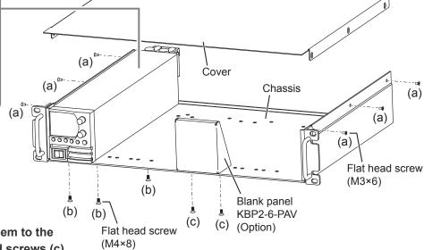
5. Attach the cover, and fix it in place with flat head screws (a).
