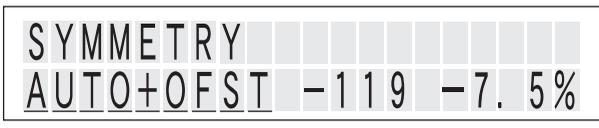
When the symmetry operation mode is set to auto or offset (AUTO+OFST), the actual slice level is displayed in percentage at the lower right corner of the screen. The peak levels of the input amplitude correspond to +50 % and -50 %.
