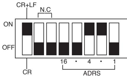
Fig.4-2 Example of setting the address to 6
