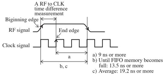
\*4.The KJM6775 has built-in FIFO memory (temporary storage memory) as waiting for calculate processing, data is acquired continuously until the FIFO memory becomes full, even if measurement of sampling period exceeds upper limit to average value: 52 MSPS to 74 MSPS. When the signal is applied at 74 MSPS, the FIFO memory becomes full at 100 data points.
