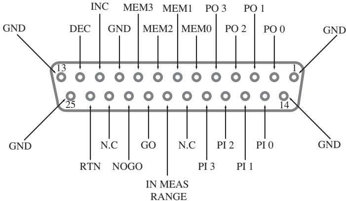
Fig.5-1 Connections of EXT I/O Connector Pins
