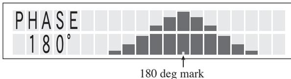
When DELAY is on, you can set the PHASE using the rotary knob.
