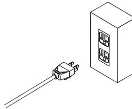
Grounded three-contact electrical outlet
