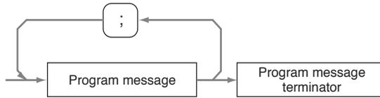
When linking program messages for send, the number of characters to be sent at any one time should be 250 characters or less, including message terminators ";", and " " (space).
