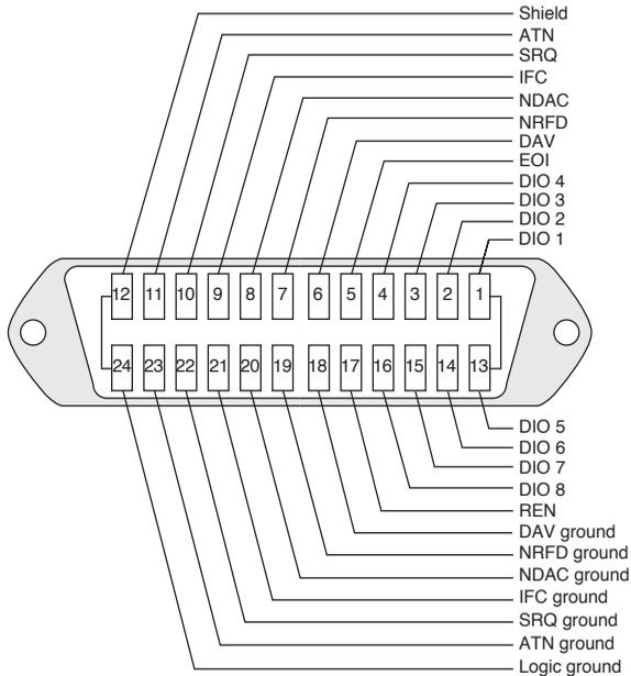
Fig.4-1 GPIB connector
