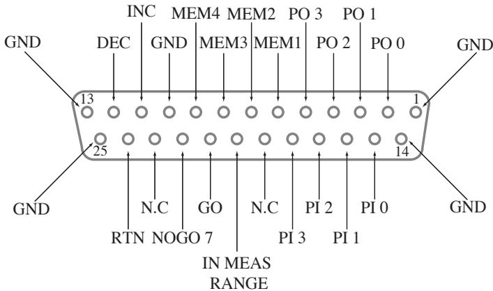
Fig. 5-1 Connections of EXT I/O Connector Pins
