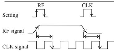
Measure the time difference between the rise of the RF signal and the fall of the clock signal and that between the fall of the RF signal and the fall of the clock signal. Then, determine the amount of jitter.
