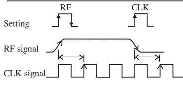
Measure the time difference between the rise of the RF signal and the rise of the clock signal and that between the fall of the RF signal and the rise of the clock signal. Then, determine the amount of jitter.
