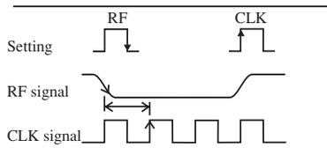
Measure the time difference between the fall of the RF signal and the rise of the clock signal. Then, determine the amount of jitter.
