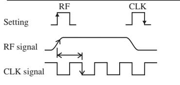
Measure the time difference between the rise of the RF signal and the fall of the clock signal. Then, determine the amount of jitter.
