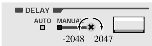
In panel operations, turning the DELAY TIME variable resistor clockwise means setting the delay in the direction of 2047, while turning it counterclockwise means setting it in the direction of -2048.
