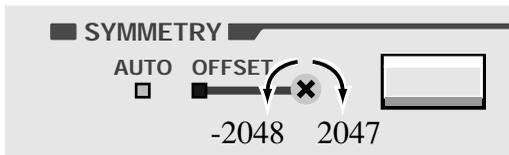
In panel operations, turning the SYMMETRY LEVEL variable resistor clockwise means setting an offset level in the direction of 2047. Turning it counterclockwise means setting it in the direction of -2048.
