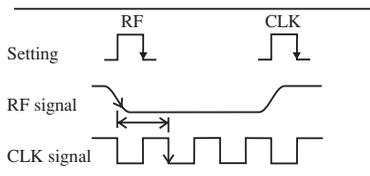
Measure the time difference between the fall of the RF signal and the fall of the clock signal. Then, determine the amount of jitter.
