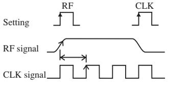
Measure the time difference between the rise of the RF signal and the rise of the clock signal. Then, determine the amount of jitter.
