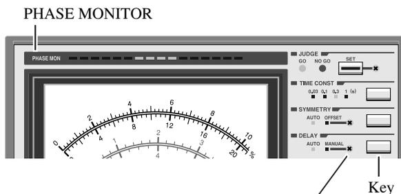
DELAY TIME setting variable register when DELAY is set to MANUAL
