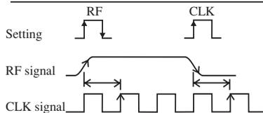
Measure the time difference between the rise of the RF signal and that between the fall of the RF signal and the rise of the clock signal. Then, determine the jitter value.
