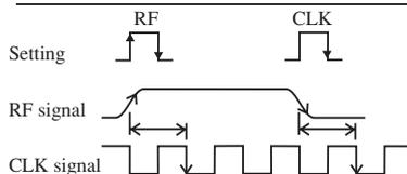
Measure the time difference between the rise of the RF signal and the fall of the clock signal and that between the fall of the RF signal and the fall of the clock signal. Then, determine the jitter value.
