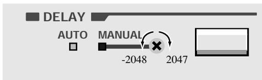
In panel operations, turning the DELAY TIME setting variable register clockwise means setting the delay in the direction of 2047, while turning it counterclockwise means setting it in the direction of -2048.
