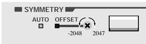
In panel operations, turning the SYMMETRY OFFSET/SLICE LEVEL setting variable register clockwise means setting an offset level in the direction of 2047. Turning it counterclockwise means setting it in the direction of -2048.
