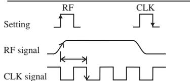
Measure the time difference between the rise of the RF signal and the fall of the clock signal. Then, determine the jitter value.
