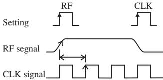
Measure the time difference between the rise of the RF signal and the rise of the clock signal. Then, determine the jitter value.
