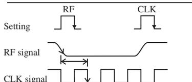
Measure the time difference between the fall of the RF signal and the fall of the clock signal. Then, determine the jitter value.
