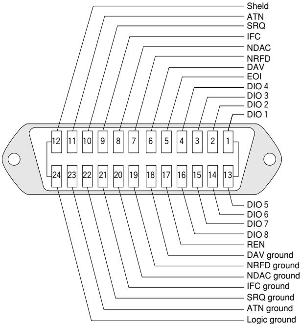
Fig. 3-3 GPIB Connector
