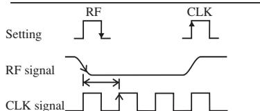
Measure the time difference between the fall of the RF signal and the rise of the clock signal. Then, determine the jitter value.
