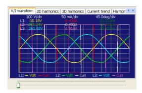
When you have set the standard to IEC 61000-3-2 Ed4.0, the class to class C, and the limit values to 3rd/5th/Current Wave, the current waveform analysis diagram that is prescribed from IEC 61000-3-2 Ed3.0(2005)/ A2(2009) is displayed in place of the V/I waveform in the test results file. (Only valid for single-phase, two-wire circuits.)
