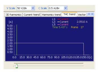
Move the cursor to the position that you regard as the maximum current value on the waveform using the track bar.
