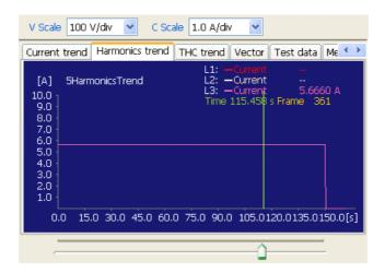
Move the cursor using the track bar while observing the current value on the waveform.
